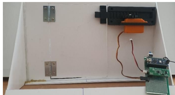
Fig. 5. Proposed access system for the technical space accessed by a passive RFID [13]
